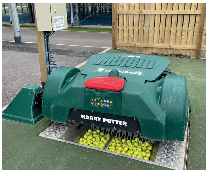
This robot can collect 400 balls an hour, and be in constant circulation operation day and night. A facility may have several robots, with each having a docking station to drop the golf balls and recharge. The advantage these machines have is that they are lighter, quieter, cost less to operate and may recharge with solar power
