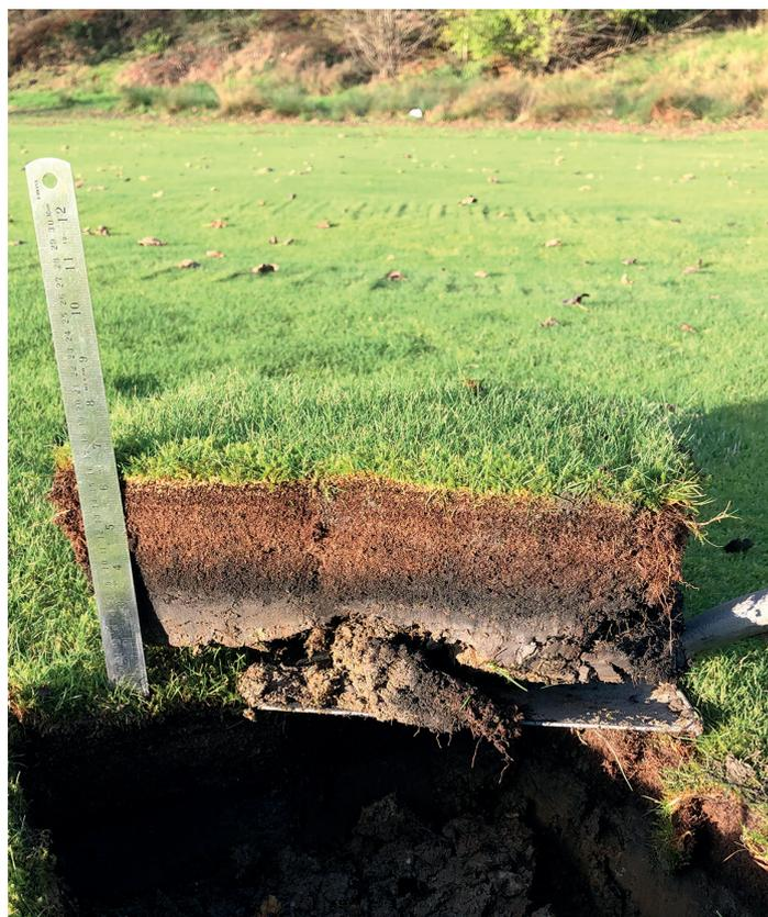
Soil and turf conditions have a direct impact on the quality of playing surfaces. This photo shows turf with an excessive amount of thatch – an undesirable surface layer of partly decomposed organic matter – which causes soft, waterlogged turf. Good golf surfaces are well drained and firm
