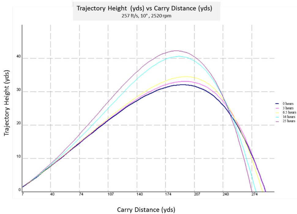
Figure 8 Effects of dimple characteristics on trajectory
