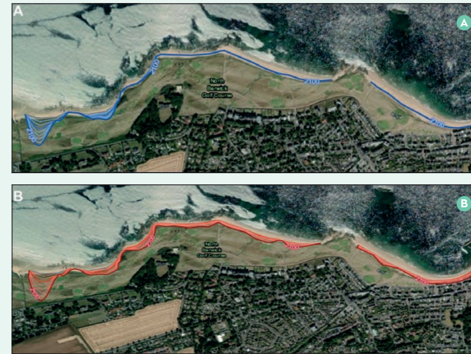
Figure 14. Estimated erosion of the coast at the North Berwick golf course 2100 based upon different emission scenarios (A) RCP2.6, 50th percentile and (B) RCP8.5, 95th percentile. Data acquired from Dynamic Coasts. www.dynamiccoast.com
