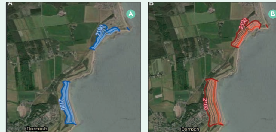
Figure 11. Estimated erosion of the coast at the Royal Dornoch golf course 2100 based upon different emission scenarios (A) RCP2.6, 50th percentile and (B) RCP8.5, 95th percentile. Data acquired from Dynamic Coasts. www.dynamiccoast.com
