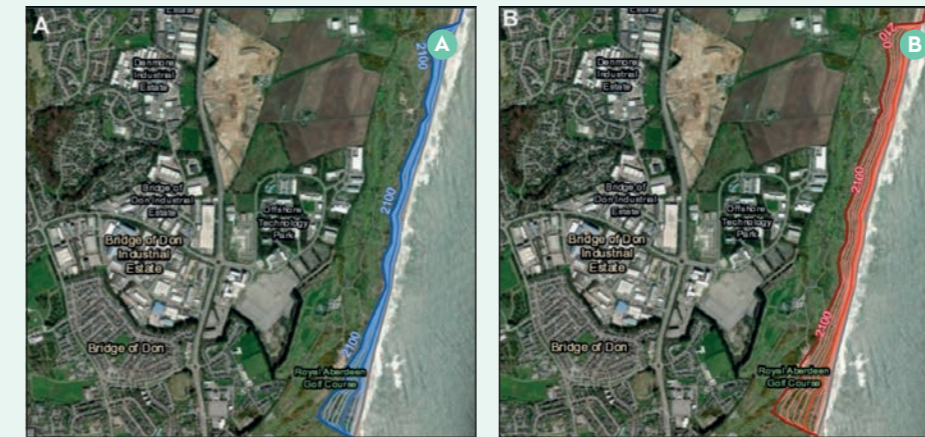
Figure 8. Estimated erosion of the coast at the Balgownie golf course 2100 based upon different emission scenarios (A) RCP2.6, 50th percentile and (B) RCP8.5, 95th percentile. Data acquired from Dynamic Coasts. www.dynamiccoast.com
