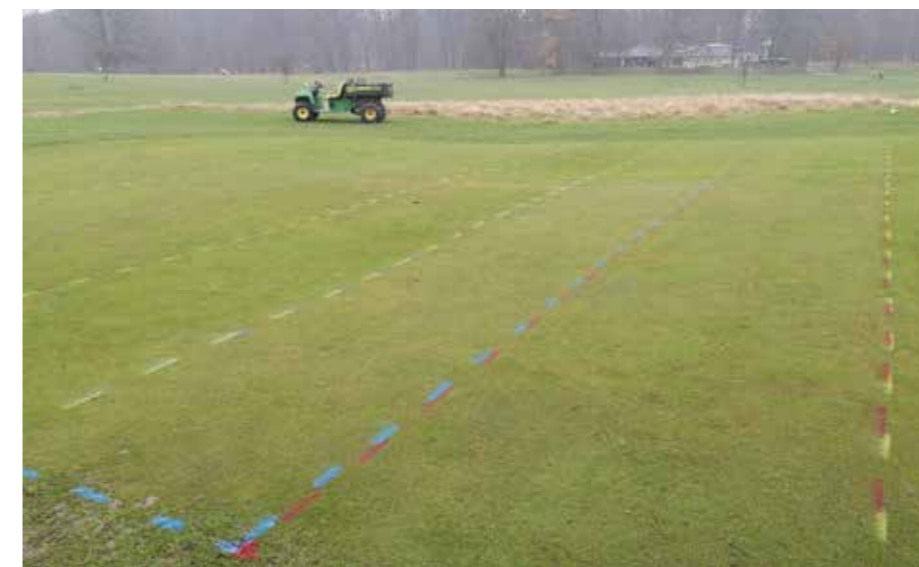
Photo 3-3: The trial area at Royal Copenhagen Golf Club in autumn 2020. From left – Yellow: No rolling; Blue: Rolled four times per week; Red: Rolled two times per week. More moss was found in plots with no rolling.
