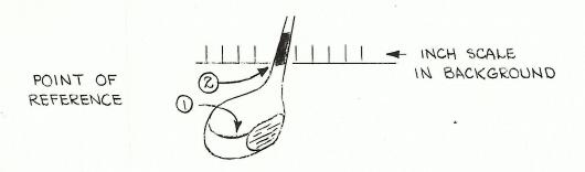
This was the only well-defined light mark on the otherwise dark clubhead. We repeated measurements of this point on the original photographs using a travelling miscroscope. (The original measurements were made with a fine scale.) These miscroscopic measurements tallied with the original ones.
