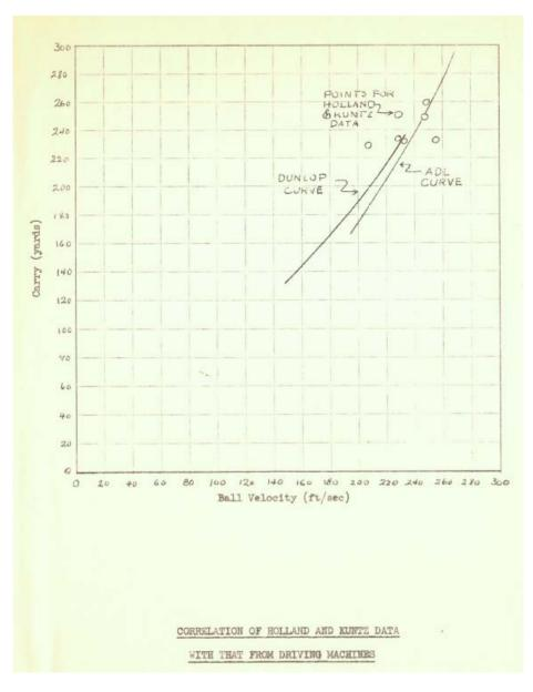
Figure 1: Carry distance vs. ball speed for Holland and Kuntz (as well as two analytical curves) .
