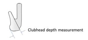
Figure 1: Definition of the clubhead depth for this test protocol.
