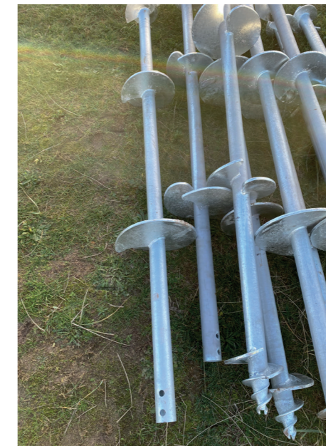
Fig A. Screw pile materials
