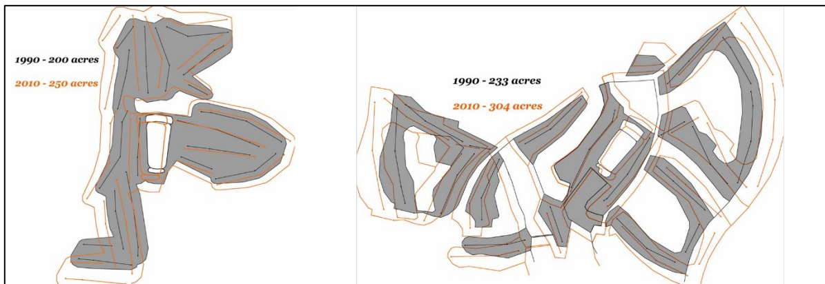
Figure 3 Effect of routing style on footprint. Contiguous style on left, residential style on right. (Bob Cupp, personal communication)
