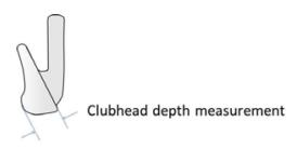
Figure 2 Definition of the clubhead depth for Section 3.c(i).
